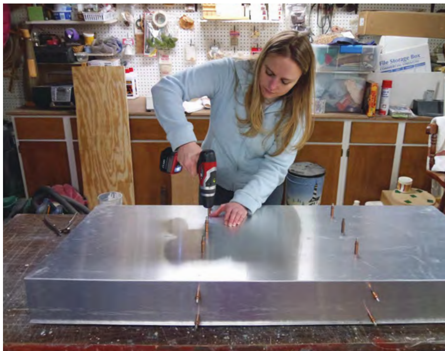
Teri works on building the center section fuel tank.
